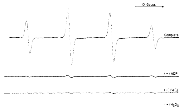
FIGURE 1: Electron paramagnetic resonance spectra of the hydroxyl free radical-DMPO spin adduct obtained in the \text{Fe(II)} -ADP- \text{H}_2\text{O}_2 system carried out as described under Experimental Procedures. The top spectrum was obtained in the complete system whereas the second, third, and fourth spectra down were obtained in the absence of added ADP, \text{Fe(II)} , and \text{H}_2\text{O}_2 , respectively. The instrumental parameters are listed under Experimental procedures.
